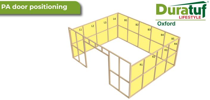
The above image shows the possible positions for PA doors. After selecting the desired position(s), use the dimensions specified in the following image to make PA door slope.
