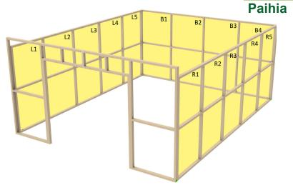
The above image shows the possible positions for PA doors. After selecting the desired position(s), use the dimensions specified in the following image to make PA door slope.
