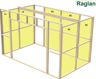
The above image shows the possible positions for PA doors. After selecting the desired position(s), use the dimensions specified in the following image to make PA door slope.
