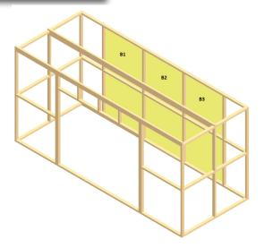
The above image shows the possible positions for PA doors. After selecting the desired position(s), use the dimensions specified in the following image to make PA door slope.
