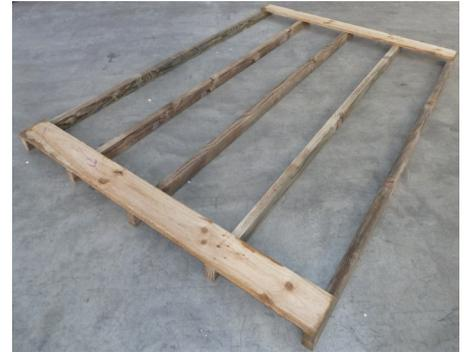
Step 2: Lay out remaining floor boards. Measure diagonals to ensure measurements are equal (i.e. floor is square). Rip down last floor board to suit gap, and nail off floor with 50mm flooring nails (12 nails per board).
