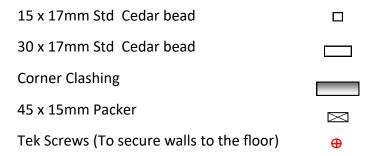
Please note: The walls are not screwed down to the floor until all the walls are erected, the roof is in place and the doors are about to be installed.
