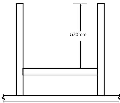
**Step 1:** Lay out the two window studs (883mm) and Nog (590mm) on a flat surface. Position Nog and nail in place using two 75mm nails at each end.
