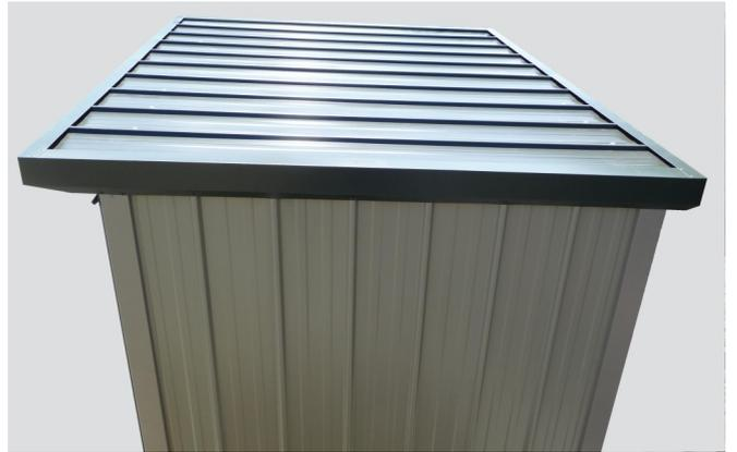
**Step 2:** Centralise Barge Flashing on end and rivet in place, one rivet into every second Rib. Fit two rivets through top of Barge into Rib. Repeat with other Barge Flashing. Check Spoutings are straight, then rivet to Roof one rivet every second Rib.
