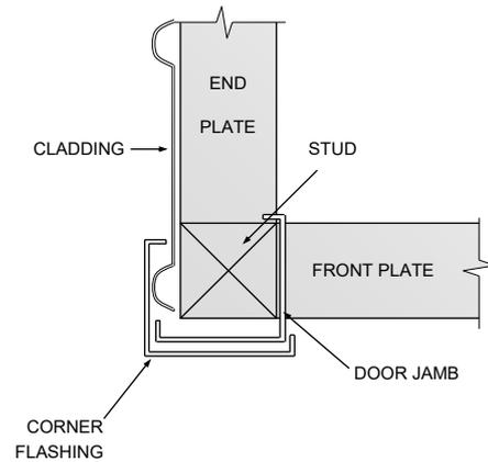
**Step 2:** On the left hand side of the front wall fit Corner Flashing (101) over Door Jamb Flashing and rib . With top of the Corner Flashing flush with the top of the Top Plate, rivet in place using six rivets.
