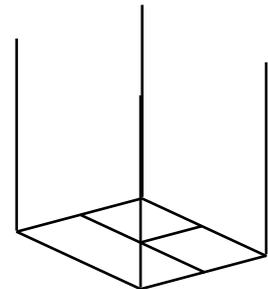
**Step 4:** Position the back wall frame on top of plates. While someone supports frame, nail in place. Nail in centre Stud using 1.205m End Wall Nogs to get correct position.
