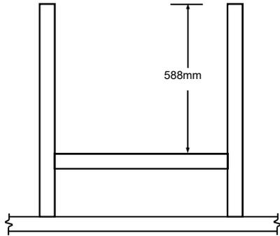
**Step 1:** Lay out the two window studs (883mm) and Nog (634mm) on a flat surface. Position Nog and nail in place using 2x 75mm nails at each end.
