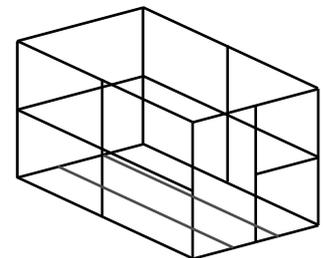
**Step 6:** Position a Jack Stud centrally on 2.545m End Wall Top Plates and skew nail in place with two 75mm nails per Jack Stud. Position Ridge Beam centrally on Jack Studs and skew nail in place using two 75mm nails each end. Pre-drilling holes before nailing will prevent timber from splitting.
