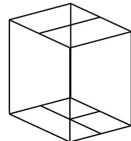
**Step 5:** Carefully roll frame over onto its base. (Pieces of timber from the packaging may be used to temporarily brace the frame before rolling it over). Position 1.205m End Wall Nogs .883m from Top Plate and nail in place. If fitting a Kiwi Floor, fit Floor Joists now. Space joists equally and nail in place using three 75mm nails per end.
