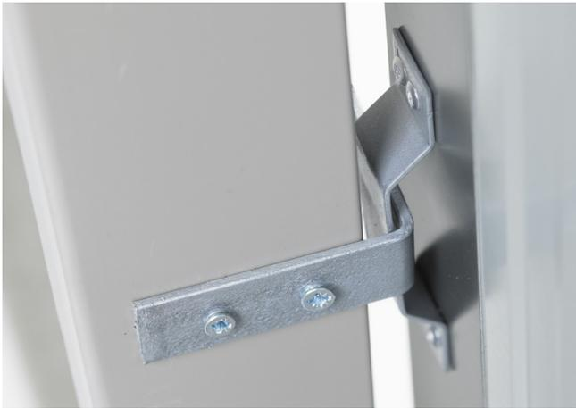
**Step 2:** Once door is hung, position the Locking Stays so they slide into the Locking Brackets easily. Screw Locking Stays to Door Jamb.
