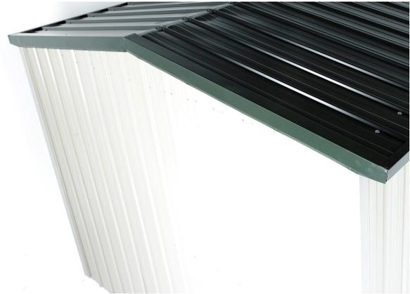
**Step 2:** Centralise Barge Flashing on gable end and rivet in place, one rivet into every second Rib. Fit two rivets through top of Barge into Rib. Repeat with other Barge Flashing. Check Spoutings are straight, then rivet to Roof one rivet every second Rib.
