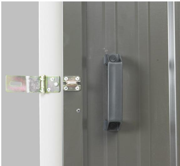
Using six rivets and one 50mm clout attach hasp to Door Jamb Flashing and the staple to the Door as shown.
