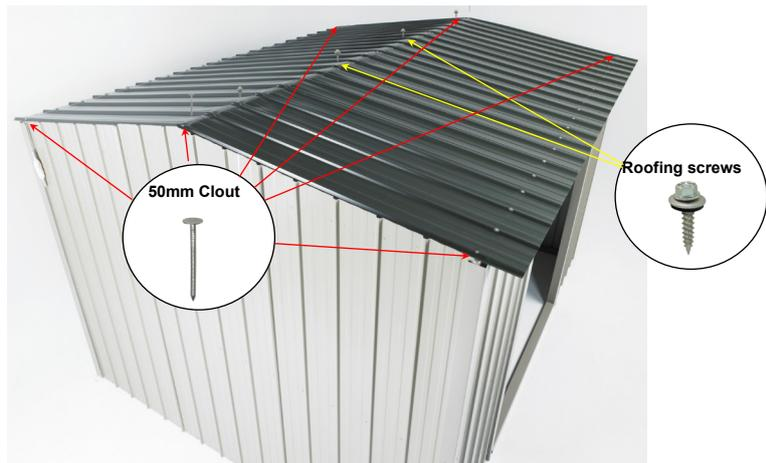
**Step 4:** Centralize Roof at the other end and nail through Rib into the Ridge Beam and Top Plates, using 50mm Clouts. Ensure Ridge Beam is straight, then Screw one 50mm Roofing Screw into Ridge Beam through each Rib on overlap (one screw per sheet). At the back, set up a String Line in centre of Top Plate. Ensure Top Plate is straight and screw, using one 50mm Roofing Screw per Rib. Repeat at the front.
