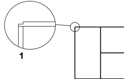
**Step 2: Front Wall:** Select one 1.715m Base Plate (Green), one 1.715m Top Plate (Red), three Studs (Yellow) and a .785m Nog. Nail studs to each end of Plates. Nail in remaining stud using .785m Nogs to get correct position. Position Nog .883m down from Top plate and nail in place.
